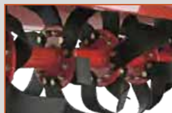
Rotor with 6 blades per flange
