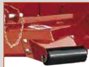
Standard front antiscaling roller
