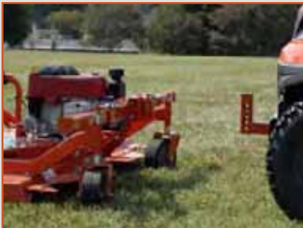
Front mount application with 2" receiver hitch
