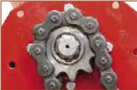
Lateral ASA 80 chain drive transmission in oil bath
