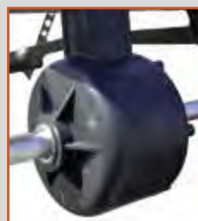
Sealed gearbox manufactured by Befco with metal gears
