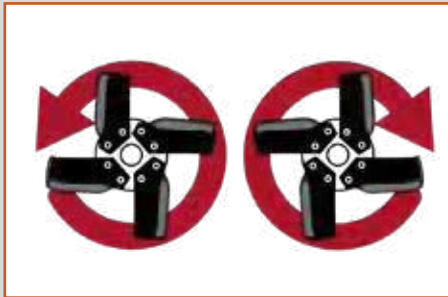
Forward or reverse tilling rotation
