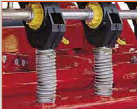
Precise seed metering cups
