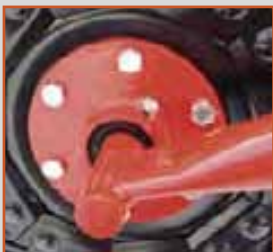
Cast steel hubs with greasable tapered bearings
