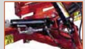
Two hydraulic cylinders with ball valves
