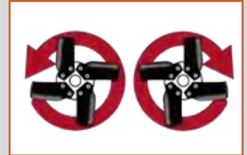
Forward or reverse tilling rotation
