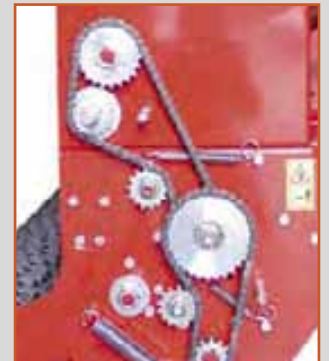
Seed distribution engaged by ASA 50 chain transmission
