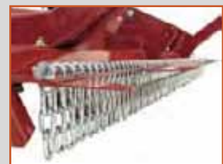
Chains provide safety from thrown objects
