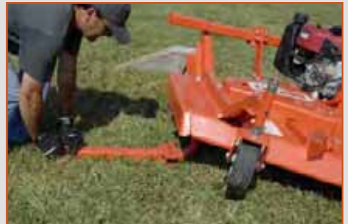
Height adjustment bar
