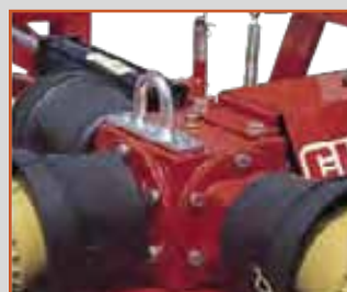
Heavy duty center-splitter gearbox
