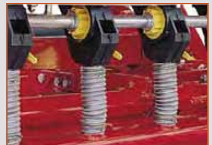
Precise seed metering cups
