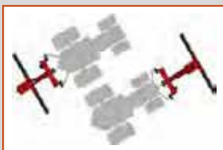
Front or rear tractor mounting
