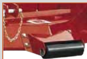
Standard front antiscalping roller
